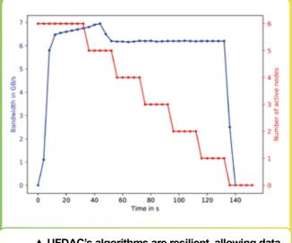
▲ UFDAC's algorithms are resilient, allowing data transfer to occur without interruption even as the number of channels, or nodes, through which information can flow become unavailable. This test allowed data to be transferred at a rate between 6 and 7 GB per second, even as the number of nodes dropped to just one. The transfer rate did not drop off until the last node shut down.
