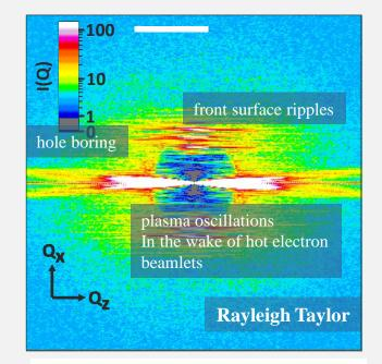
Param.:  $a_0=10$ , n=100 n<sub>c</sub>, Z/A=1/2, no preplasma XFEL 8 keV, 10<sup>10</sup> phot., focused to 5x5  $\mu$ m
