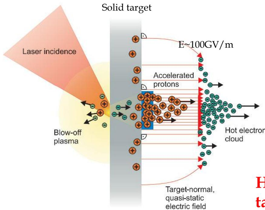
Very thin solid Hydrogen target should be interesting to produce protons beams of high energy.
