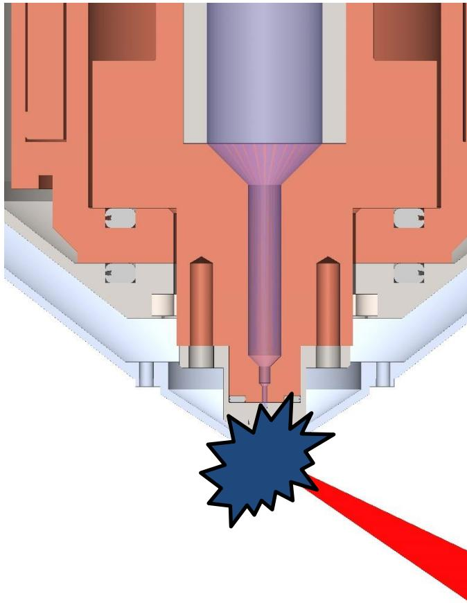
The heat generated by the hot plasma makes the temperature of the cell increase and this causes the emptying of the cell. DATA are required to design a nozzle for high frequency shot
